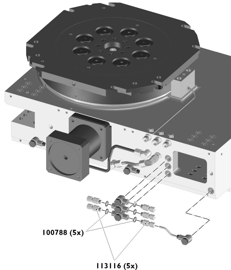
**Schleifschlitten X-Achse Chariot porte-meule axe X Grinding slide X-axis**
