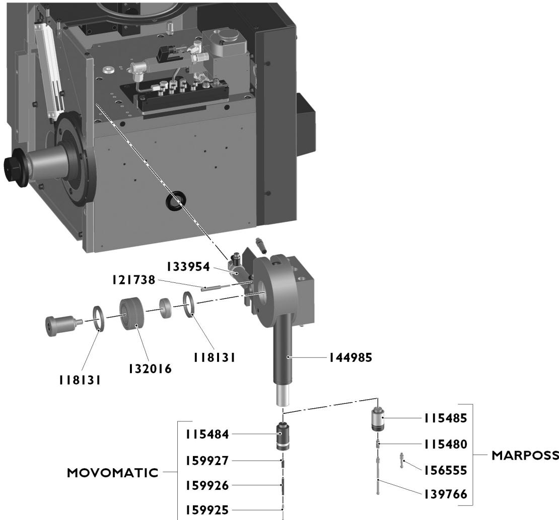
**7.19 Messsteuerung pneumatischer Rückzug Autocalibrage rétraction pneumatique In-process gauge system pneumatic retraction**
