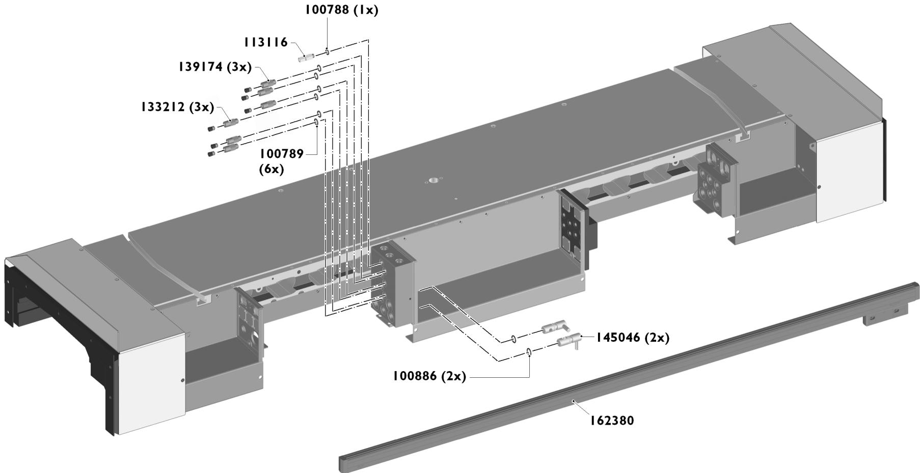
**Längsschlitten Obertisch Chariot longitudinal table supérieure Longitudinal slide upper table**
