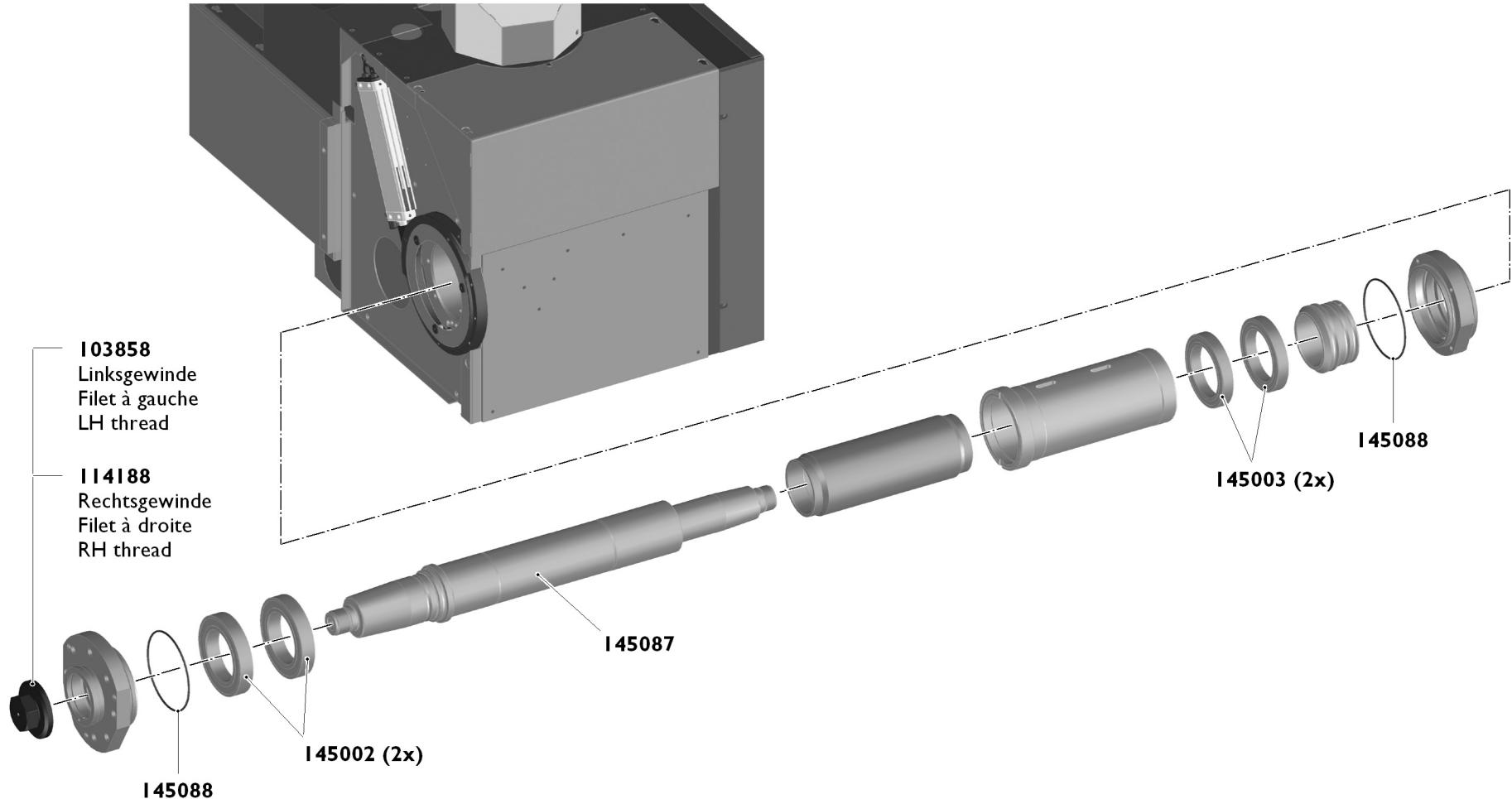
**Schleifkopf Aussenschleifen    Poupée porte-meule rectification extérieure    Wheelhead O.D. grinding**
