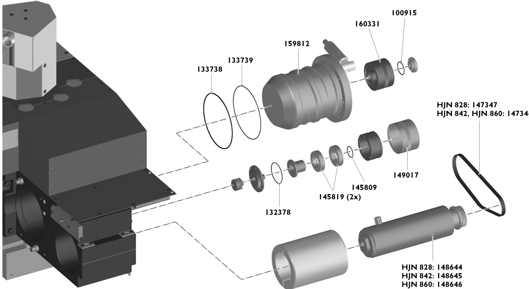
**Schleifkopf Innenschleifen Poupée porte-meule rectification intérieure Wheelhead I.D. grinding**
