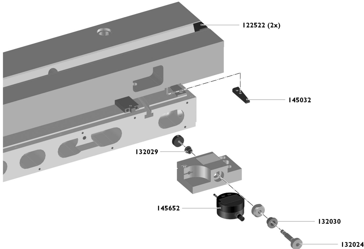
**8.2 Schleifschlitten X-Achse Chariot porte-meule axe X Grinding slide X-axis**
